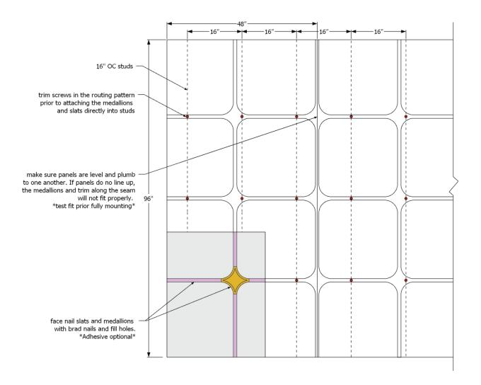
Alternate installation: MF375 Monarch Z-Clips can also be used to attach panels to wall. Slats and medallions will still need to be face nailed to the panels.
